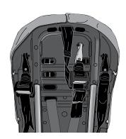
1. Disconnect Tether **Hook and Lower Anchor Hooks** from the back of the child restraint.
