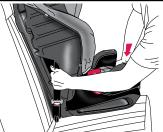
5. Remove all slack from the seat belt. Using your full weight, push the child restraint firmly into the vehicle seat while tightening the seat belt to remove excess slack.
