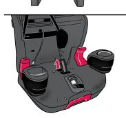
Pull the anchor through the seat and adjust so it lies flat, as shown.
