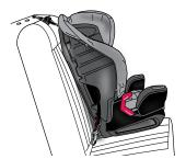
**DO NOT** install by this method for a child weighing more than 20.4 kg (45 lbs).
