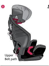
5. Push the chest clip and buckle tongues through the upper belt path to the back of the child restraint.
