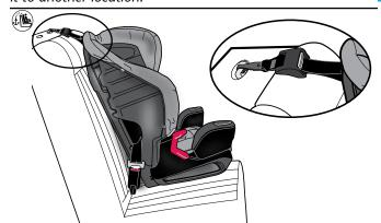
8. Connect and tighten Tether Strap.
