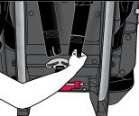
3. Remove both harness straps from the splitter plate on the back of the child restraint.
