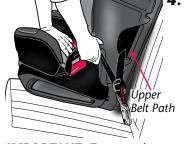
**IMPORTANT:** To properly secure this child restraint, it **MUST NOT** move more than 25 mm (1 inch) from side to side or from front to back at the upper belt path. If you can not tightly secure the child restraint, try again, move it to another location, or install with vehicle seat belt.
