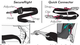
Refer to your vehicle owner's manual to locate the lower anchor bars on your vehicle seat. Attach the right hook, or clip, to the right anchor bar and the left hook, or clip, to the left anchor bar. Double check that the lower anchor connector hook is fully engaged by pulling hard on the lower anchor connector strap. Make sure vehicle seat belt lies flat without twisting.
