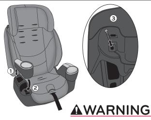
Cup holders **MUST** be installed before use of this Child Restraint.
