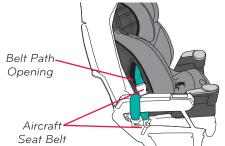
**2.** Route aircraft seat belt through belt path. Route the aircraft seat belt through the belt path opening in the back of the child restraint and continue through the opening on the opposite side of the child restraint.
