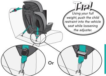
Tilt and slide the adjuster to loosen.
