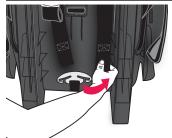
2. Remove both harness straps from the splitter plate.
