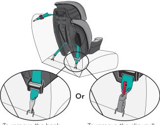
To remove the hook, press the tab and twist, then remove from anchor. To remove the clip, pull the red release strap and remove clip from anchor.
